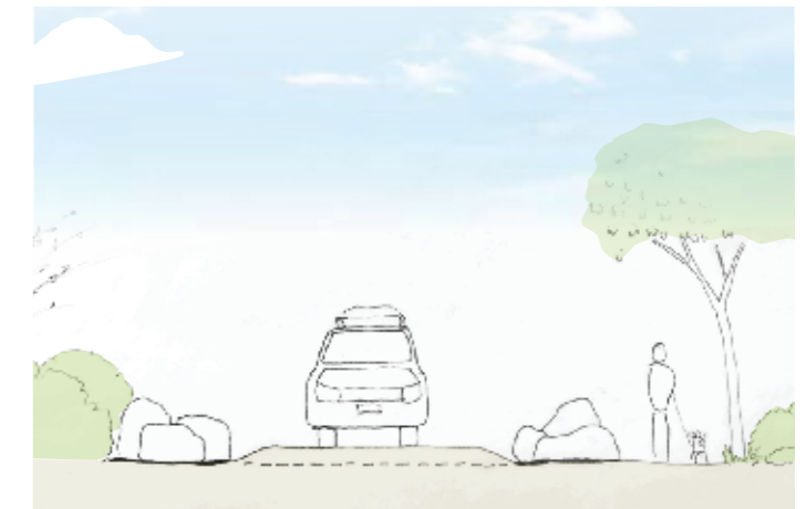
Figure 19: illustrative image of speed hump with rockwork and adjacent footpath
