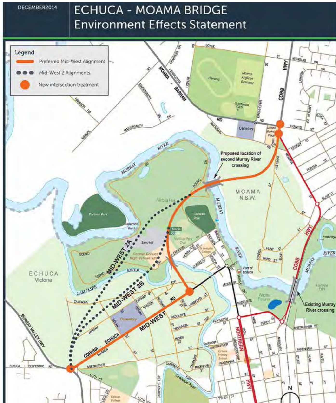
Figure 13: Plan showing alternative alignments of Echuca-Moama Bridge Project. Image source: VicRoads
