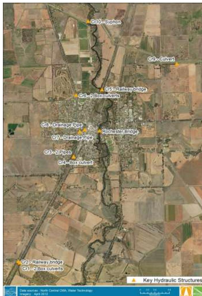
**FIGURE 3-3 LOCATION OF MAIN HYDRAULIC STRUCTURES**
