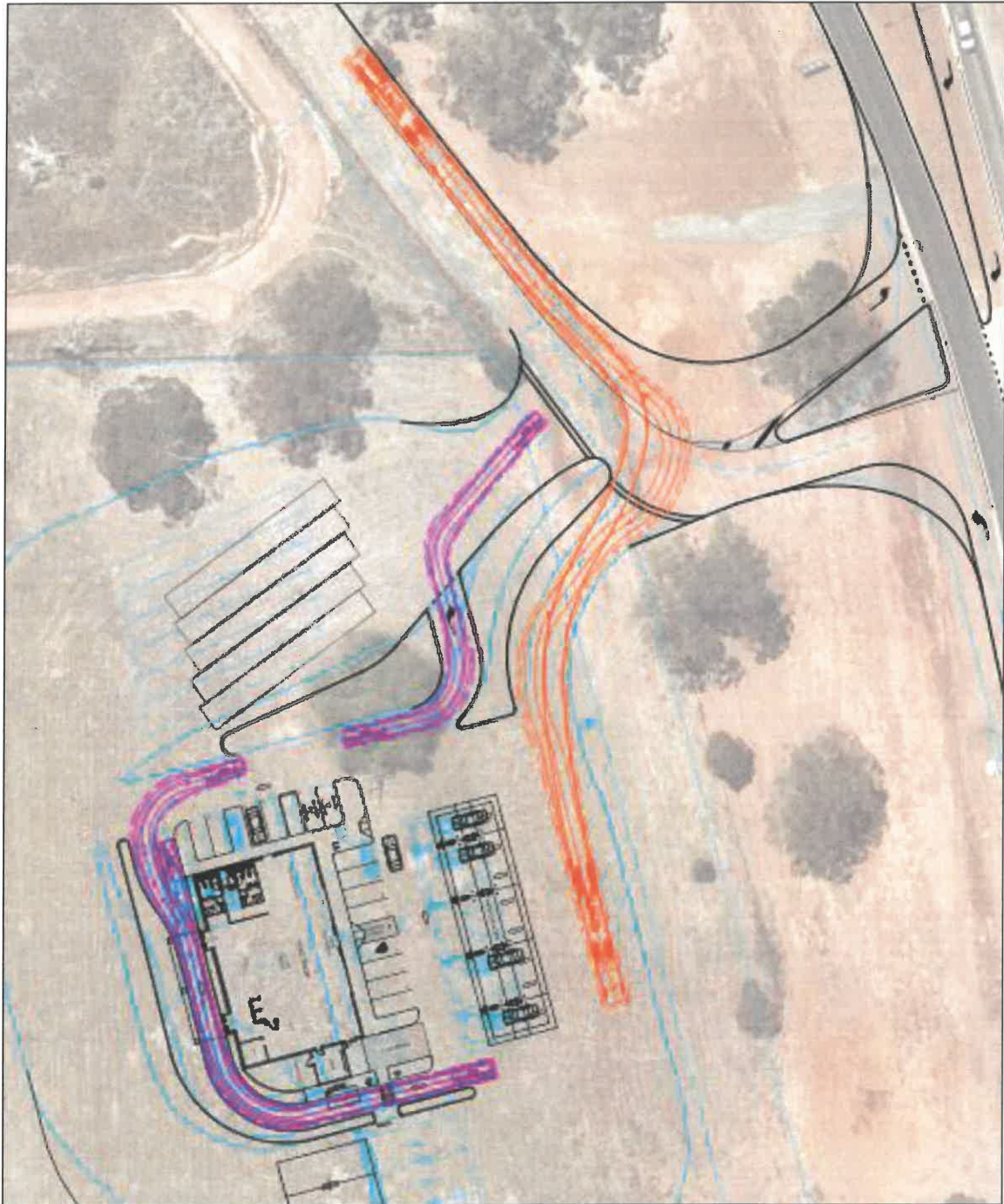
Figure B4: Circulation through drive-through by car and entry from service road by semi-trailer
