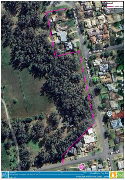
Figure 5-10 Haverfield Street Levee
