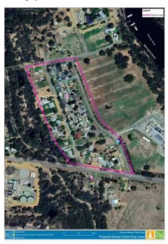
Figure 5-2 Bynan Street Modelled Ring Levee
