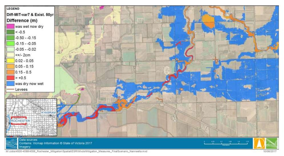
FIGURE 8-8 DIFFERENCE PLOT FOR THE 2% AEP EVENT, COMPARISON BETWEEN EXISTING AND MITIGATED CONDITIONS (NANNEELLA DEPRESSION)
