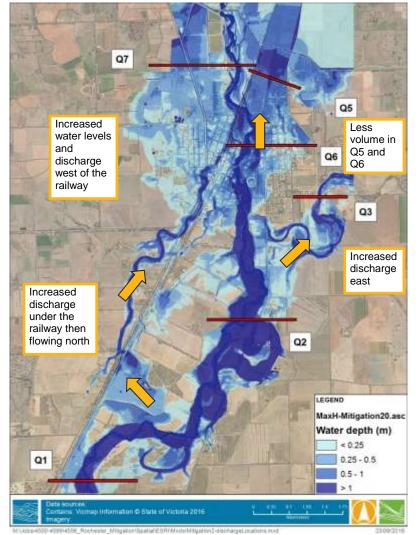
Q1: the same design events are used for modelling; therefore, the upstream inflow is identical (855 m<sup>3</sup>/s, calculated as a check)
