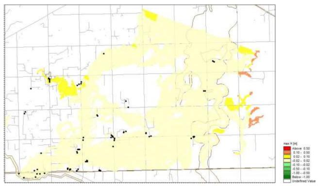
FIGURE 7-9 IMPACT OF INITIAL PONDING. DIFFERENCE PLOT ON WATER LEVELS ALONG THE NANNEELLA DEPRESSION, DOWNSTREAM OF THE WARANGA CHANNEL CROSSING.
