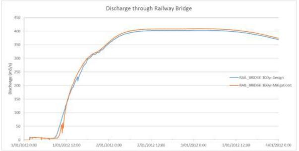
FIGURE 4-7 DISCHARGES THROUGH THE ROAD AND RAILWAY BRIDGES UNDER DESIGN AND MITIGATION CONDITIONS
