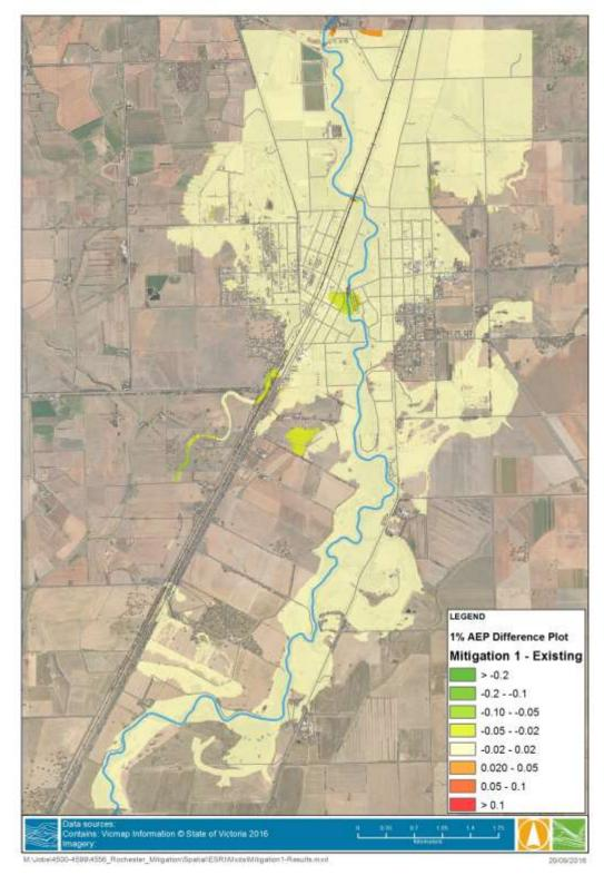
FIGURE 4-8 DIFFERENCE PLOT OF WATER LEVELS OBTAINED AFTER IMPLEMENTING THE MITIGATION OPTION (INCREASED CAPACITY OF HYDRAULIC STRUCTURES). NEGATIVE VALUES INDICATE LOWER WATER LEVELS ASSOCIATED WITH THE GREATER FLOW CAPACITY OF THE STRUCTURES.
