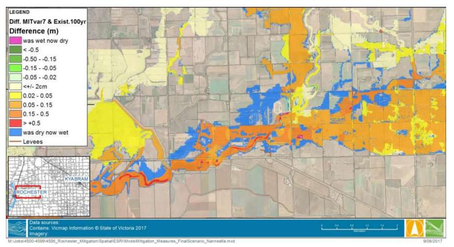
FIGURE 8-7 DIFFERENCE PLOT FOR THE 1% AEP EVENT, COMPARISON BETWEEN EXISTING AND MITIGATED CONDITIONS (NANNEELLA DEPRESSION)
