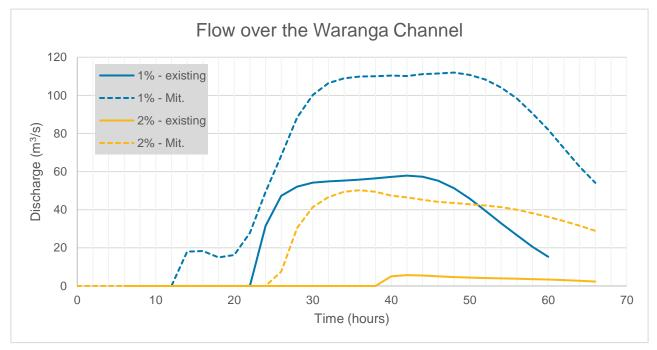
FIGURE 8-6 DISCHARGE OVER THE WARANGA CHANNEL SIPHON
