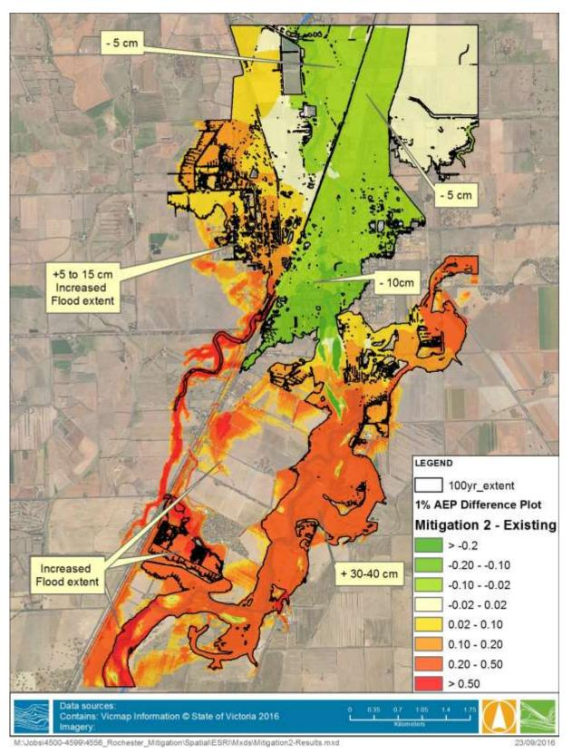
FIGURE 4-5 DIFFERENCE PLOT OF EXISTING AND INCREASED ROUGHNESS CONDITIONS. NEGATIVE VALUES INDICATE LOWER LEVELS WITH AN INCREASED ROUGHNESS. THE BLACK CONTOUR SHOWS THE FLOODING EXTENT UNDER EXISTING CONDITIONS
