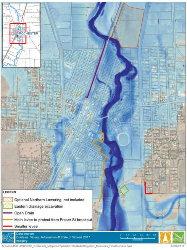
FIGURE 7-1 KEY FEATURES OF THE SCHEME TO BETTER ENGAGE THE EASTERN DRAINAGE LINE
