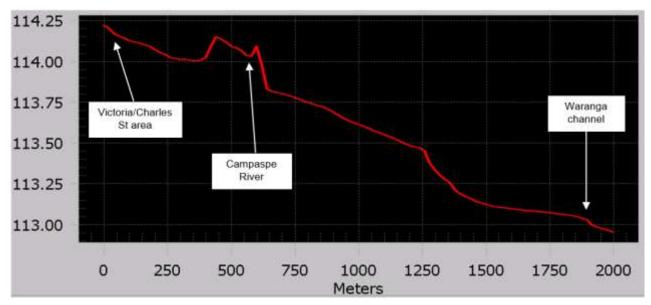
FIGURE 11-2 CROSS-SECTION 1 OF 1% AEP WATER LEVELS BETWEEN ROCHESTER AND THE WARANGA CHANNEL TO THE WEST OF THE RAILWAY LINE
