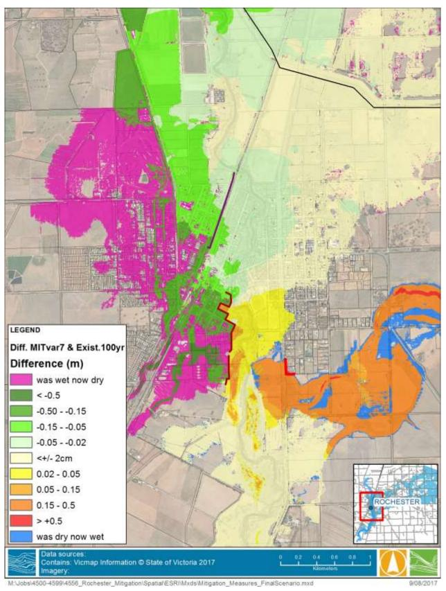
FIGURE 8-4 DIFFERENCE PLOT FOR THE 1% AEP EVENT, COMPARISON BETWEEN EXISTING AND – MITIGATED CONDITIONS (ROCHESTER)
