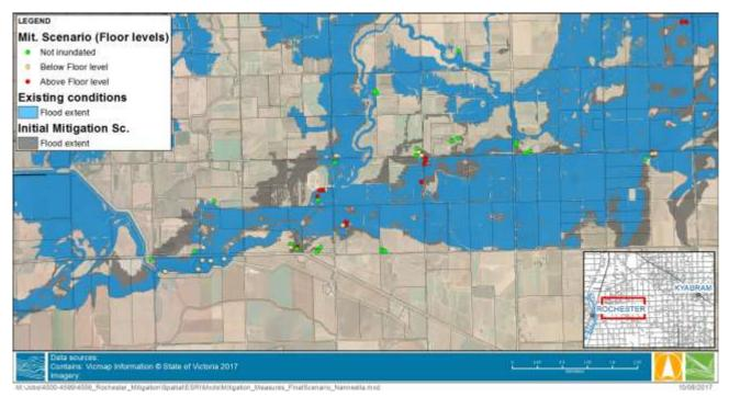
FIGURE 7-2 FLOOR LEVEL SURVEY AND IMPACT ON FLOODING OF RE-ENGAGING THE EASTERN DRAINAGE LINE
