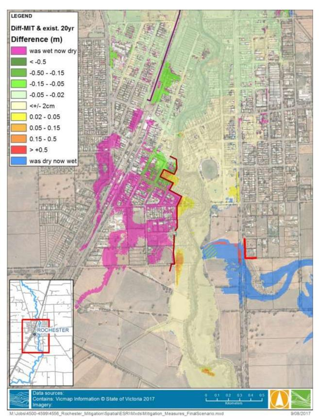
FIGURE 8-5 DIFFERENCE PLOT FOR THE 5% AEP EVENT, COMPARISON BETWEEN EXISTING AND – MITIGATED CONDITIONS (ROCHESTER)
