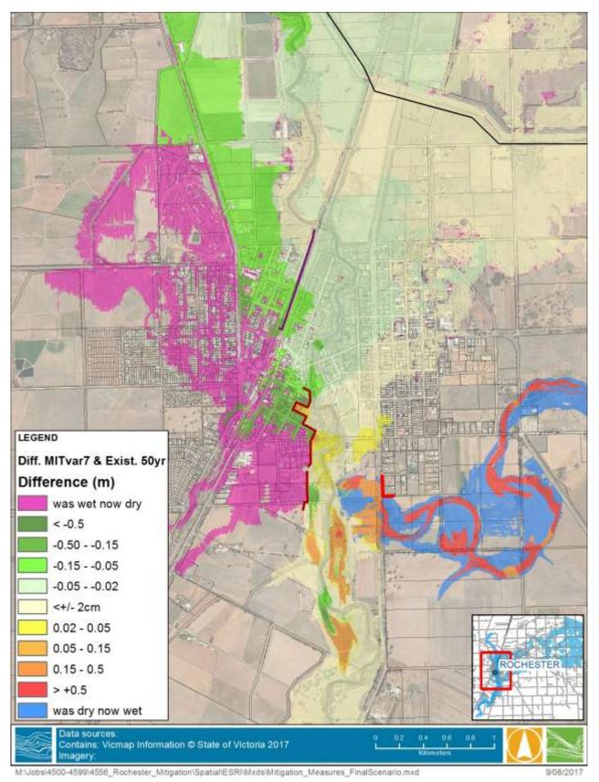
FIGURE 8-3 DIFFERENCE PLOT FOR THE 2% AEP EVENT, COMPARISON BETWEEN EXISTING AND – MITIGATED CONDITIONS (ROCHESTER)
