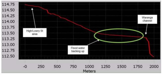
FIGURE 11-4 CROSS-SECTION 2 OF 1% AEP WATER LEVELS BETWEEN ROCHESTER AND THE WARANGA CHANNEL TO THE EAST OF THE RAILWAY LINE
