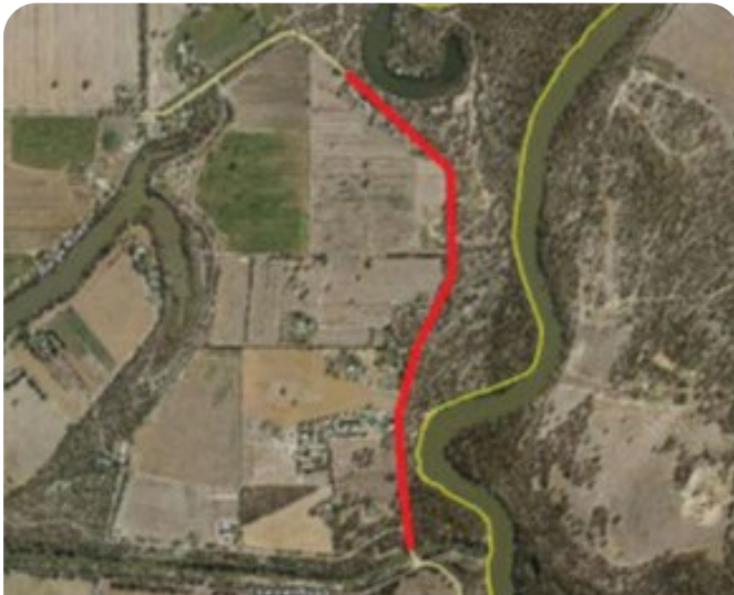
Section of levee being removed from Headworks Road
