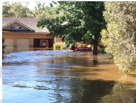
Figure 6: 1 Star Standard of Service - Inundation of dwelling or commercial or industrial premises, water greater than 300mm above floor level in a 1% AEP event.
