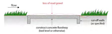
Figure 9 BT9 Addition of Concrete Floodway
